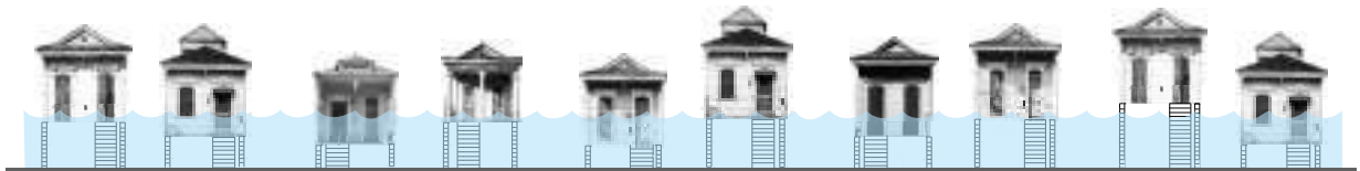
flooded streetscape of homes elevated to BFE and higher (3 to 8 feet)
