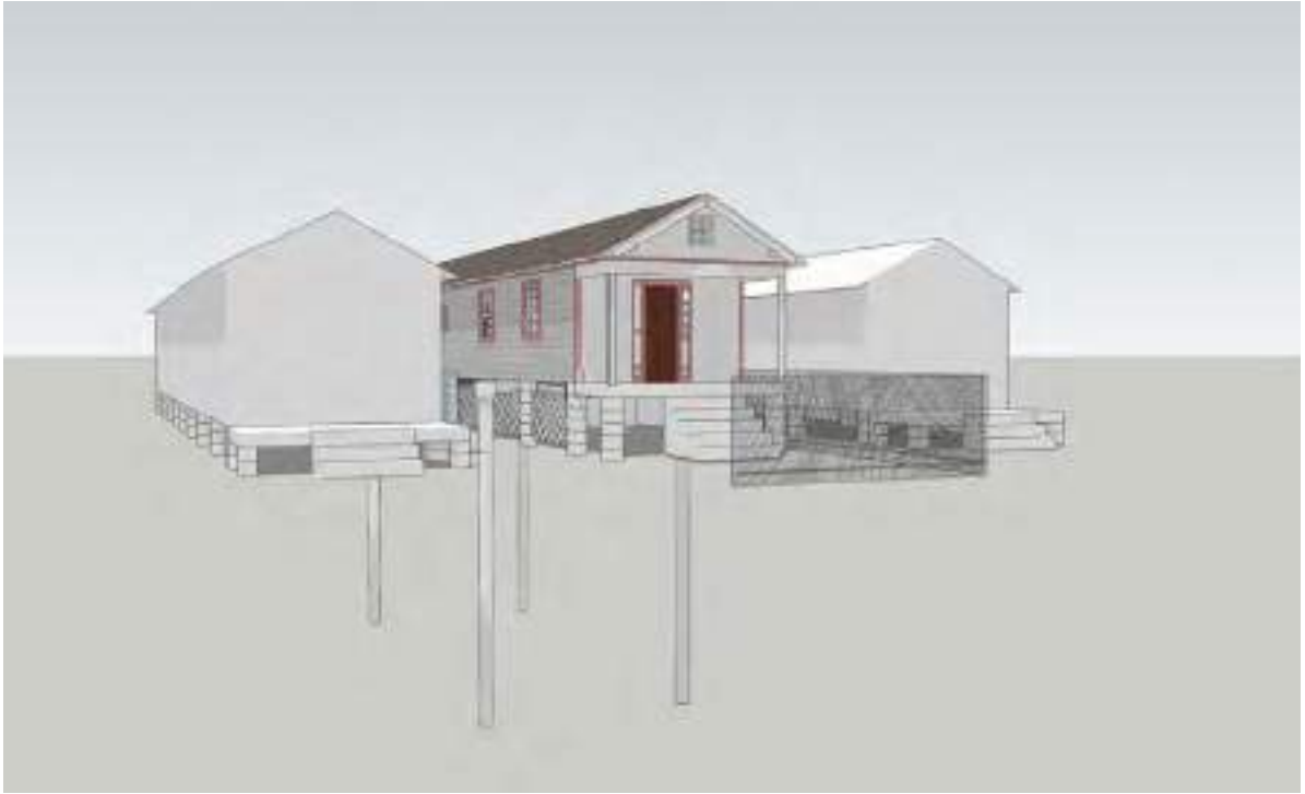
fig. 97: Conceptual Rendering of 1315 Lamanche Street Retrofit with the Buoyant Foundation System
