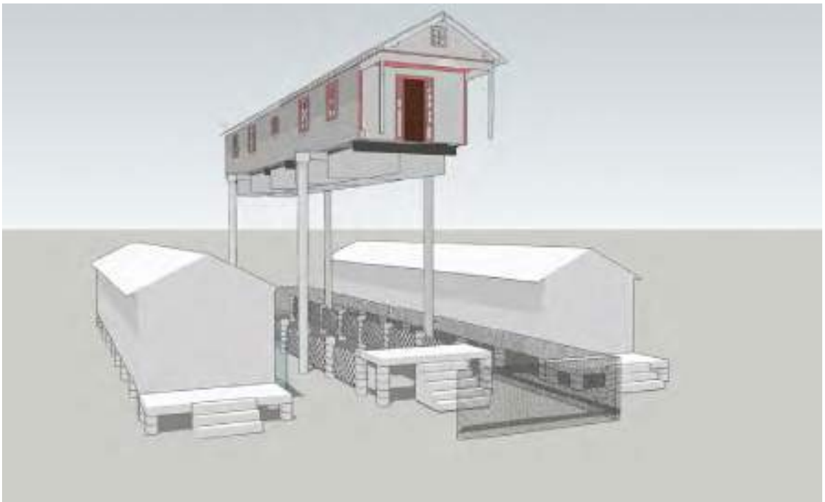
fig. 98: Conceptual Rendering of 1315 Lamanche Street Retrofit with the Buoyant Foundation System, Fully Extended
