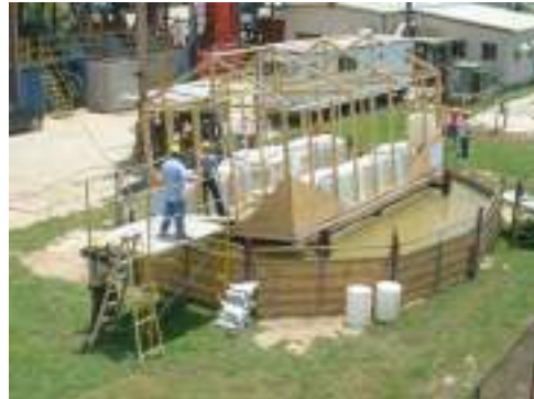
Moving the sandbags to tilt the house
