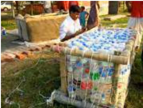
Buoyancy blocks made of recapped empty plastic bottles
