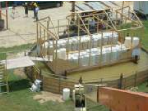
Water barrels and sandbags are added to simulate weight of house and its contents
