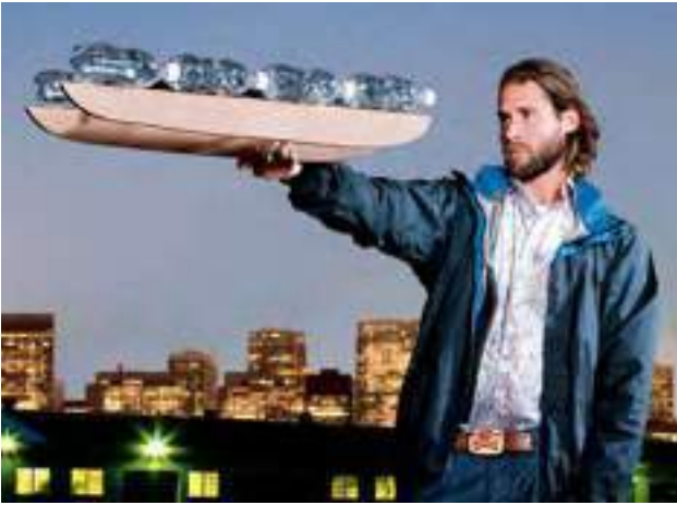
fig. 239: Plastic Water Bottles Used for Flotation
