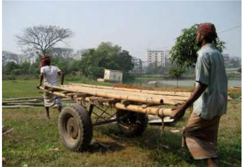
8.43. Bamboo delivery on a “Thelagari”, a vehicle made of bamboo, wood, and two tires pulled by two men
