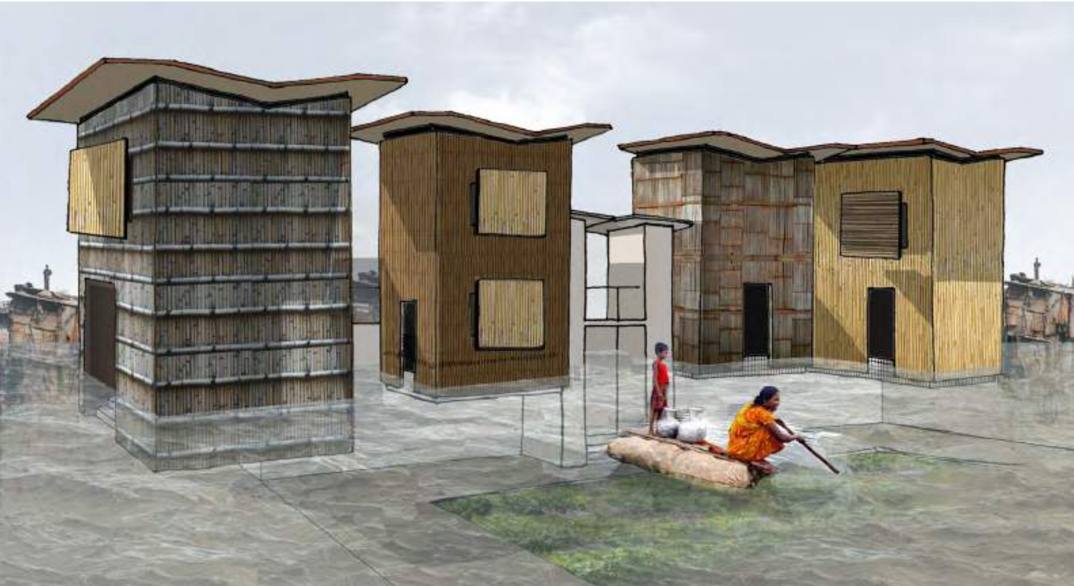
6.8. Amphibious houses floating in a LIFT community during a flood
