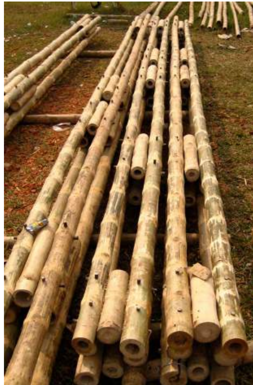
7.13. Prefabricated bamboo columns for the LIFT house
