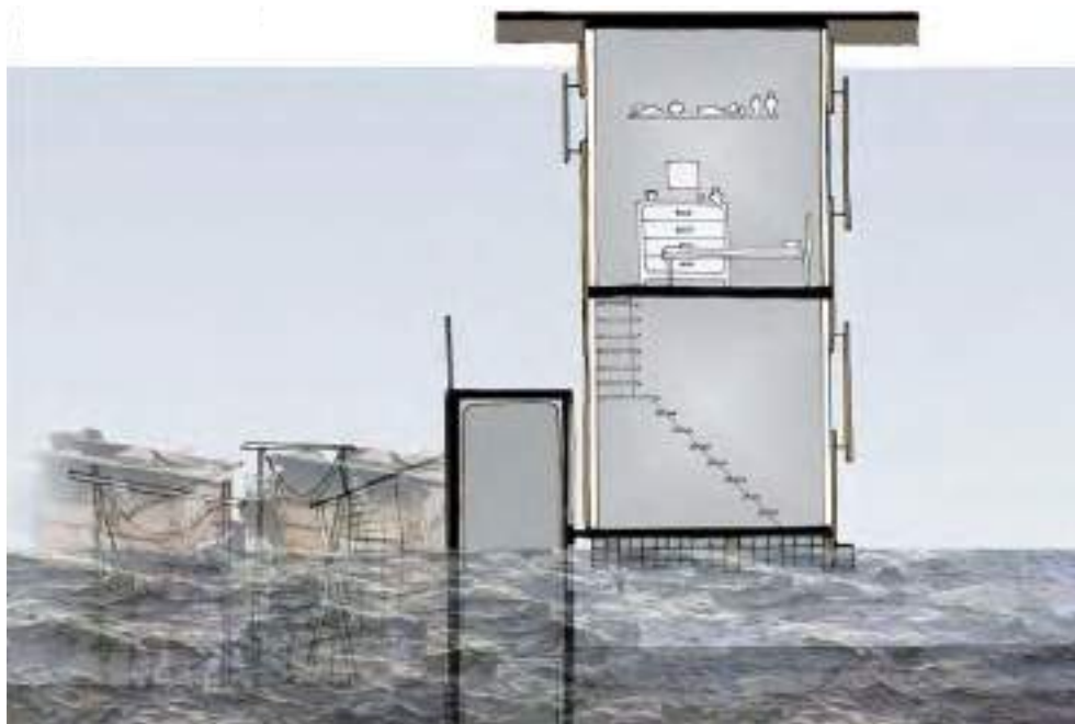
6.4. The LIFT house floating on water during floods
