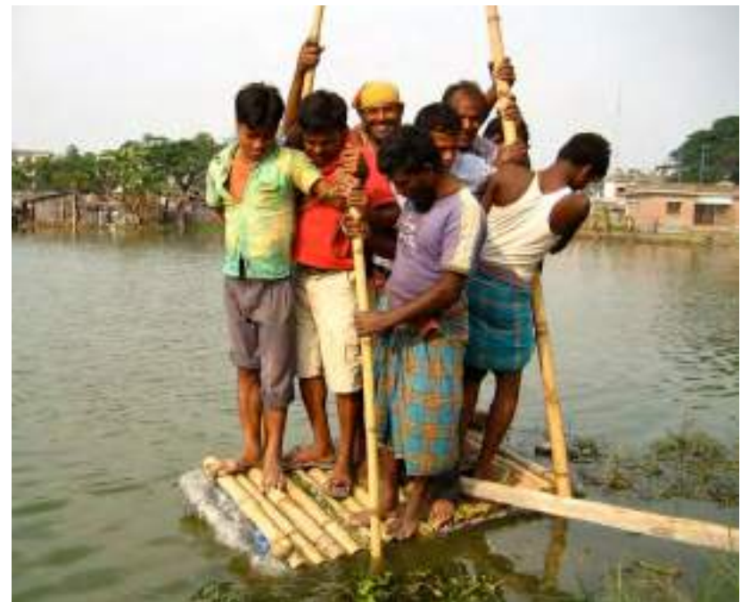
8.37. Workers testing the water bottle foundation model for live load capacity
