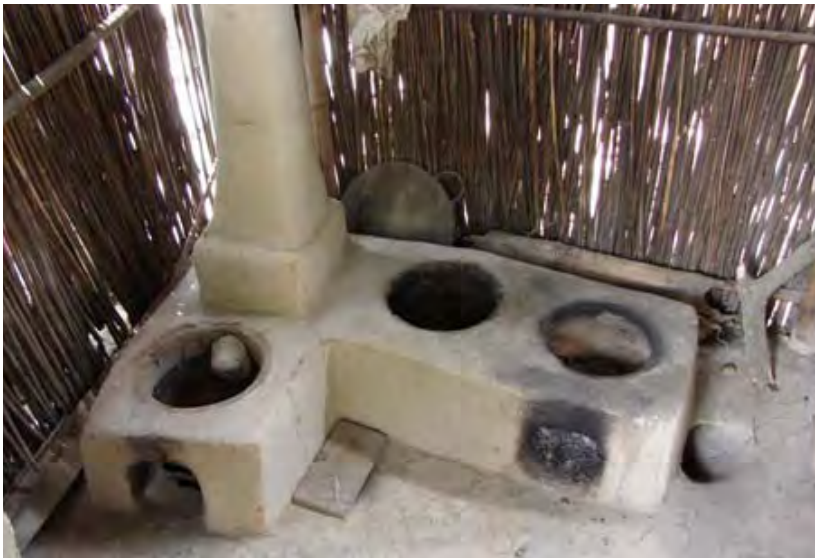
7.12. Improved stove with an exhaust chimney
