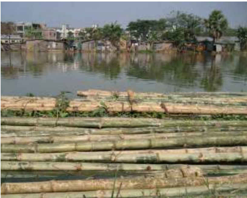
8.46. Bamboo treated in the traditional method of submerging in a water body
