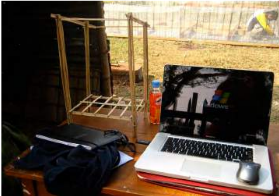
8.68. Stick model of bamboo dwelling to communicate to bamboo workers
