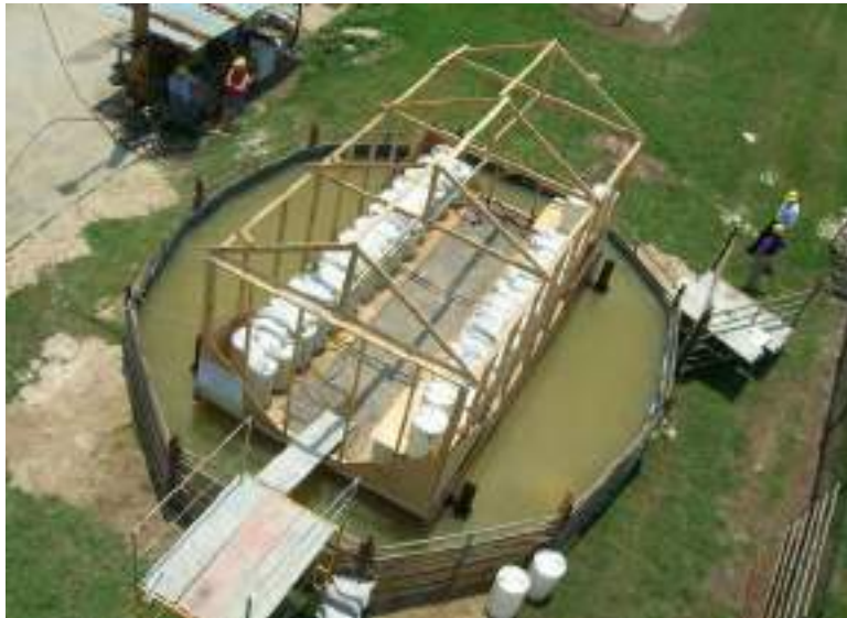
5.11. LSU prototype demonstrating floatation of amphibious structure
