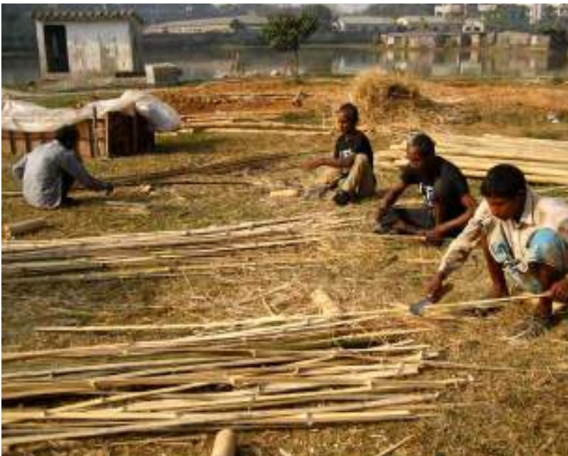
8.119. Mulli bamboo split for facade finish
