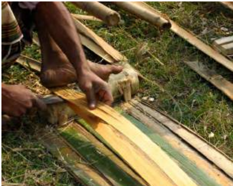
8.87. Special blade used to split Mulli bamboo into thin strips
