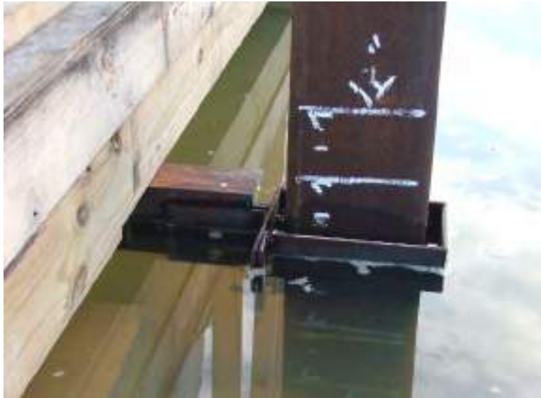
5.10. Vertical guidance system for the LSU prototype
