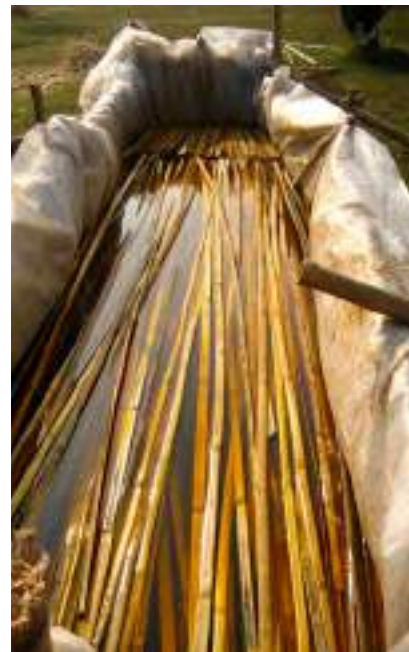
8.121. Treatment of bamboo for facade finish
