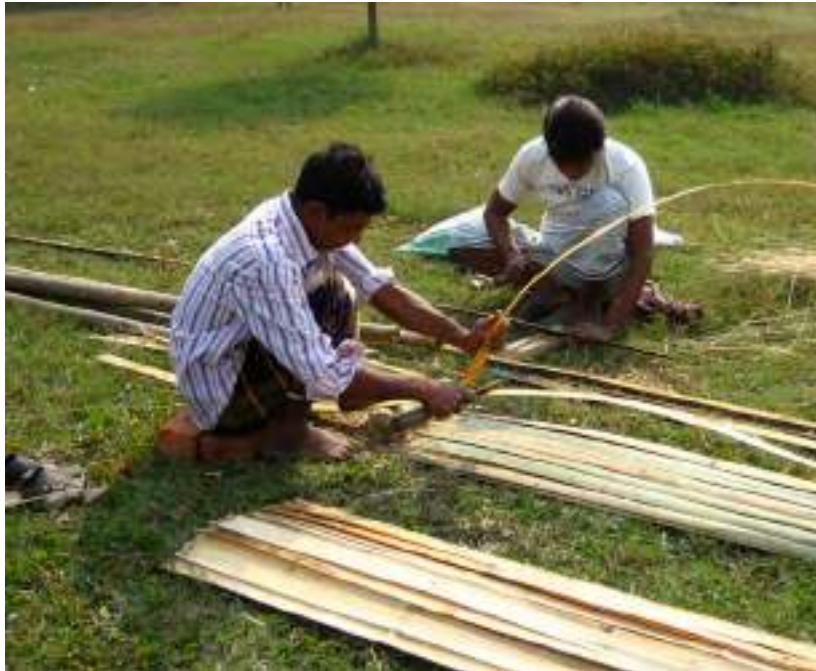
8.86. Mulli bamboo split into thin strips for weaving
